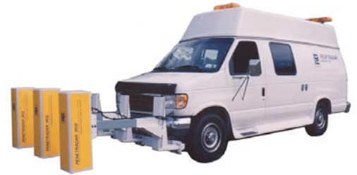
Standard IRIS Vehicle shown with 3 Model 30AGC Antennas
