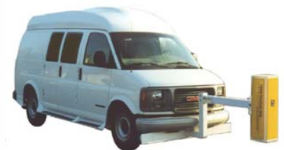
Basic IRIS Vehicle Installed with one Model 30AGC antenna
